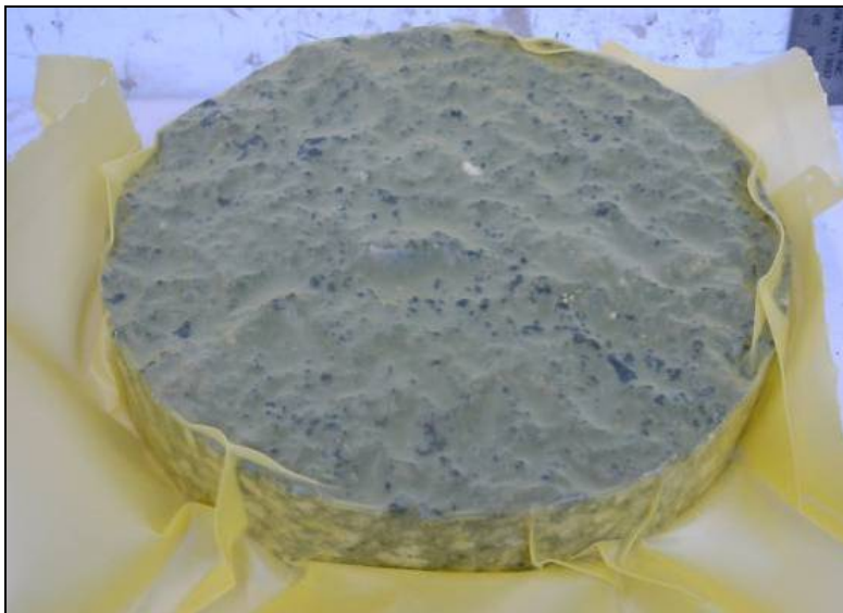
Figure 24: CoreLok seal of specimen.
