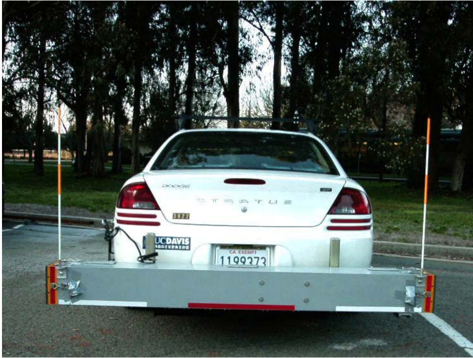
Figure 22: Laser profilometer beam.
